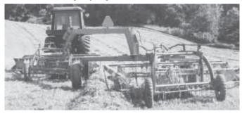
A lengthened Hesston 1024 hydra swing frame pulls a left and right hand rake at the same time.
