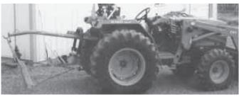
Rail hangs from 3-pt. mounted posthole auger frame so it's easy to get into comers.
