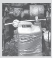
A 16-in. long plastic toilet supply line, inserted through lid, serves as spout to pour chemical into oiler.
