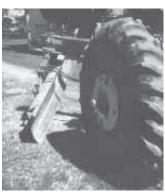
Robert Rodenberg tips blade to steepest angle and drops front end into ground about 2 ft. from post. Before blade gets to post, he raises it to pull post out.
