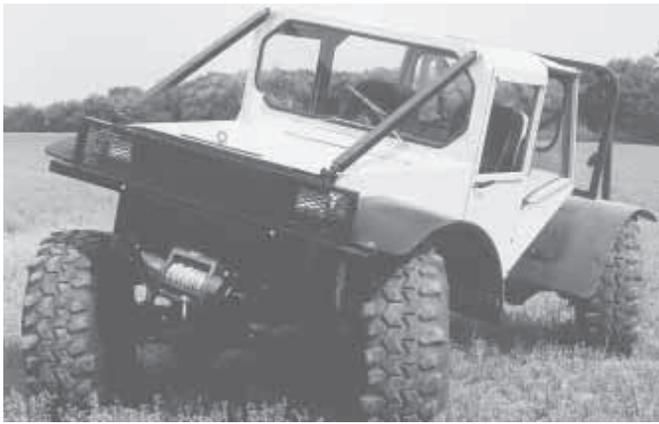
"Sidewinder" has crab steering, a body supported by a computer-controlled air bag suspension system, a wheel base that extends on-the-go, and a homemade cab with a pair of air-cushioned seats in front.
