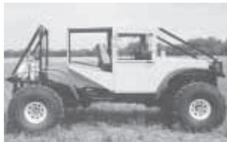
Home built "ATV" is powered by a Chevy Vortec engine connected to a 700 R4 transmission.
