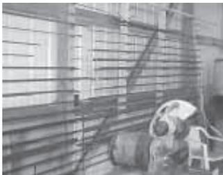
quantity of many sizes of steel on hand. To use space efficiently, I built this rack onto the walls of my shop. In 24 ft. of wall space, I have room for 48 sizes of stock. I made the racks simply by drilling upward tilting holes in the 4 by 6 posts and the 2 by 4 studs in between. I then drove 10-in. sections of 3/8-in. dia. rebar into the holes. The rebar was a lot cheaper than big spikes would have been."
