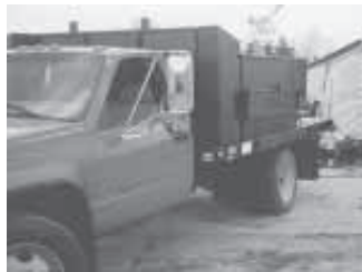
Lee Schunk's 1999 Chevy 3500A 1-ton pickup is equipped with a 12-ft. flatbed. On each side are toolboxes that measure 4 ft. long, 4 ft. high, and 2 ft. deep.
