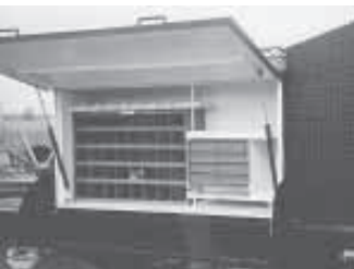
Doors on each toolbox are hinged at the top and swing out, with help from a pair of gas shock assist cylinders.
