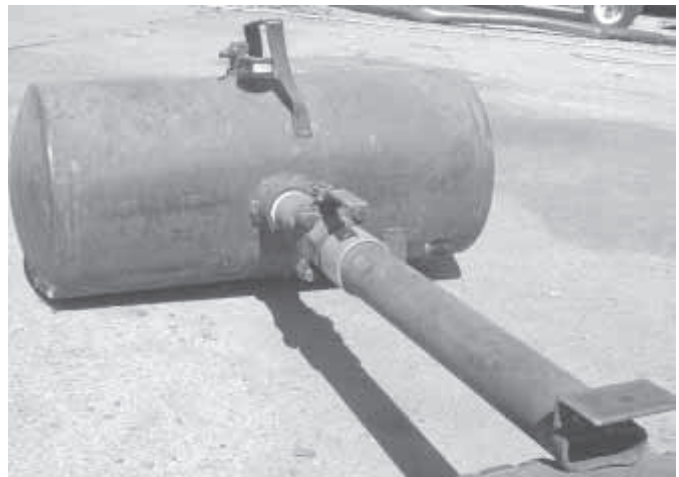
Brian Maring's tire bead seater consists of an 8-gal. air tank and a large butterfly valve that lets all the air out at once.
