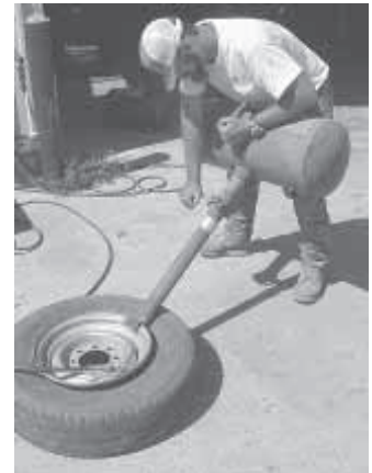
To seat tire bead, you fill tank with air and then rest angle iron piece against rim so pipe points between tire and rim.
