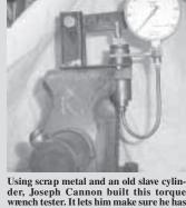
der, Joseph Cannon built this torque wænch tester. It lets him make sure he has just the right pressure on a bolt head.
