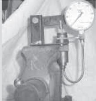
**Using scrap metal and an old slave cylinder, Joseph Cannon built this torque wrench tester. It lets him make sure he has just the right pressure on a bolt head.**
