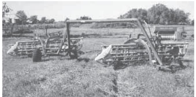
Kutzler built this gooseneck hitch and two-wheeled rear dolly. "It lets me pull two 9-ft. rakes at a time and cover twice as much ground at virtually no extra cost," he says.
