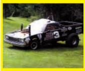
wheel drive car is equipped with a 327 cu. in., 8-cyl. engine that I souped up to about 500 hp, and it has a 3-speed manual transmission. I installed new exhaust headers, a new dual carburetor, and a new rear end. It has won several local awards in the "doodlebug" class at local contests, and took second place last year in the 5,000-lb. pulling class where it pulls a weight transfer sled weighing 17,000 lbs. (Russell Adams, 1956 Five Mile Square Rd., Island Pond, Vt. 05846 ph 802 723-4790)
