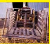
I use old pallets to make wood racks to haul firewood. Each rack measure 5 ft. square and is made from three pallets. They stand about 1 ft. above ground so I can slip a pair of bale prongs under them using my IH 560 tractor. Some of
