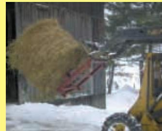
Spinner attaches to loader arms and is used to pick up bale.
