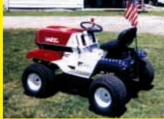
could fix it. I first decided to paint it and, as you can see, I got a little carried away. Then I extended both rear axles and the front spindles. I put big tires all around and made front fenders out of rear fenders from another tractor. I got the 10 hp. motor running and then read an article in FARM SHOW about someone who made a little tractor that ran 45 mph. So I changed pulleys on the transaxle and on the motor so that this little tractor now runs 45 mph and even does wheelies.
