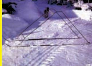
I made this ski walker to support my bum leg. I bolted old wooden skis to a 1 in. wide by 1/2 in. cold rolled steel piece that makes the skis a few feet longer. The frame is a 3/8 in. steel rod welded to each end of the skis to stabilize it. It's good exercise and makes walking on ice easier. (Gordon J. Brietzke, R.R. 1 Box 26 S 4, Spirit River, Alta. T0H 3G0).
