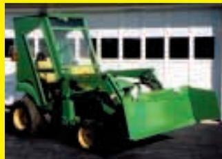
I used angle iron and 1/2-in. plywood to make the cab and plexiglass for the windows. The angle iron frame bolts to the tractor's roll bar using existing holes in the roll bar. Foam rubber fills the space
