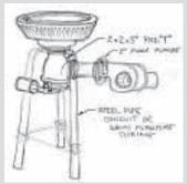
Pickup brake drum mounted on tripod stand is all you need to make a simple forge.
