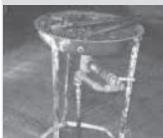
Compressed air plumbed into bottom of fire pot keeps fire hot.
