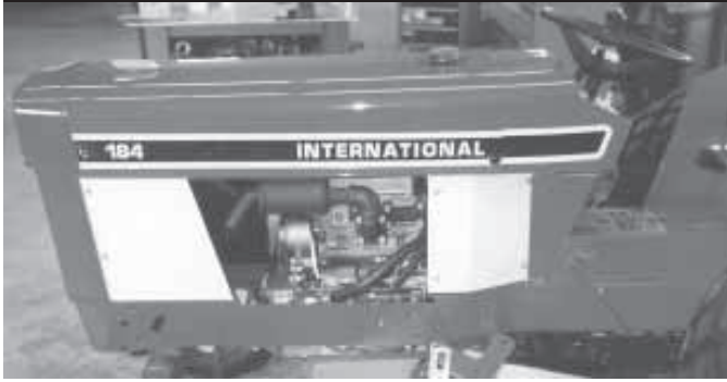
New Yanmar 3-cyl. diesel engine fits into Cub 184 and cost Mike Schnoebelen about $2,300.
