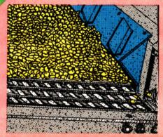
New grain-saving deflector prevents grain build-up along combine sidewalls to eliminate grain loss on sloping as well as level ground.
