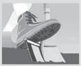
magazine. You can give your shovel-shoving foot a more comfortable pushing surface by cutting a slit in a scrap of 1-in. pvc pipe and slipping it over your shovel's flange. If it won't stay put, just add a bead of hot-melt
