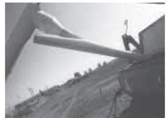
Max Serr used a 6-ft. piece of 4-in. pvc pipe to make a simple auger spout that he uses to load bulk seed into his drill.
