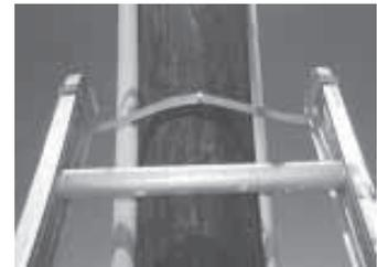
Safety device consists of a spring metal strap with a box-shaped bracket at each end that slips over top rails of extension ladder.
