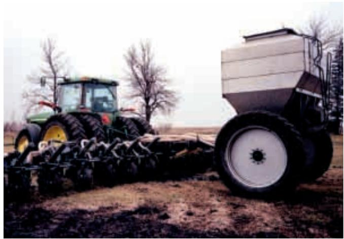
High capacity fertilizer caddy "steers" itself to precisely follow in the tracks of any implement. Two-wheeled unit is designed primarily to deep band granular fertilizer, but can also be used in any row crop application, liquid or dry.
