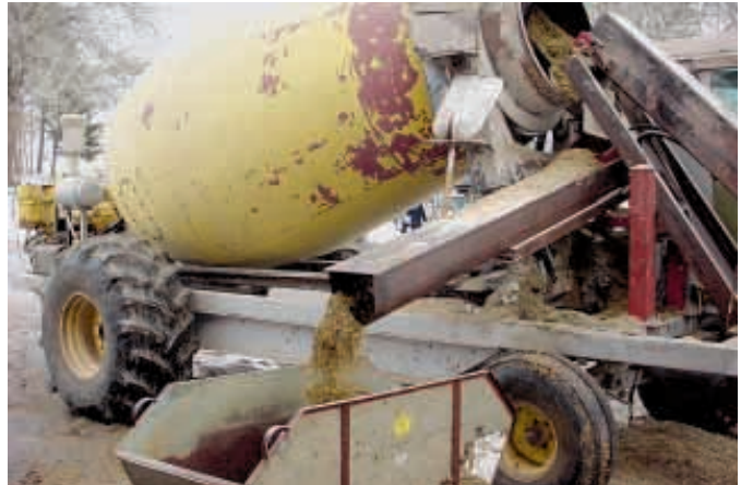
Unloading auger tilts down close to bunk or feed cart so wind doesn't blow feed away.
