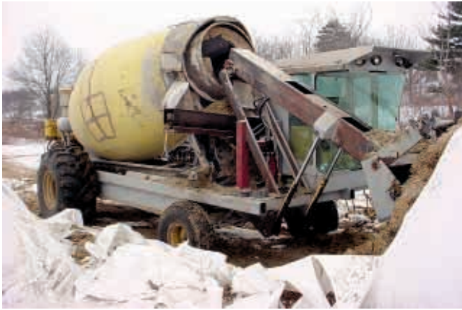
Dave Retzlaff built this self-propelled TMR mixer from parts off a combine and cement mixer. Photo above shows front view of mixer being loaded.
