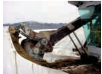
Home-built mechanical "mouth" tears away silage at face of silage bags and feeds it into elevator.
