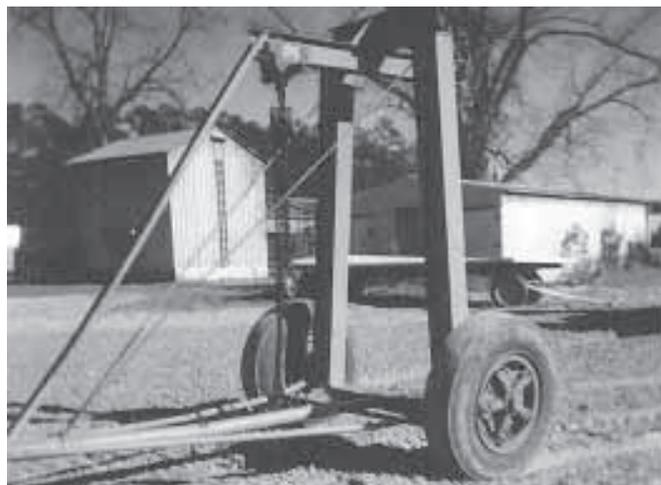
Frame and wheels are from a large truck's front end. Van Arnette added 8-in. I-beams from a scrap yard, and a 2 1/2-ton hoist and chain.
