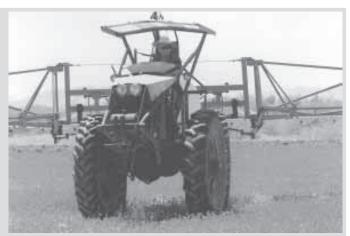
Lightweight homemade sprayer has articulated steering, 4-WD and tractor tires.
