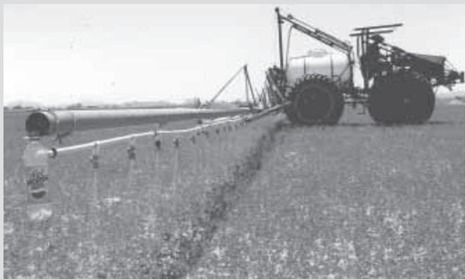
Pendulum-mounted boom is so delicately balanced that pumping water between soda bottles at each end of 100 ft. boom helps balance it.
