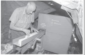
Harvey Severson feeds blocks of wood into the Severson Shaver, which turns a tray of wood into a big pile of wood curls in seconds.
