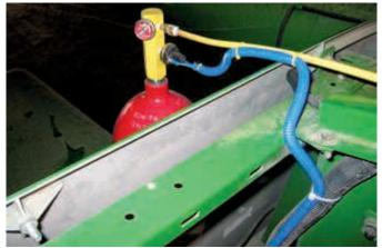
When a fire starts, cap melts off and dry chemical agent discharges out opening to extinguish fire. At the same time, a low pressure switch on system sends a signal to cab, which turns on a warning light and sounds a buzzer. Automatic extinguisher also works on clothes dryers (below).
