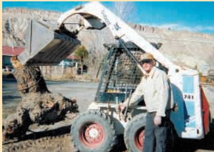
Glen Farmer added external controls for every control on his Bobcat skid loader, so he can maneuver it without having to crawl in (above). He cut a hole through the undercarriage frame on the left side of loader and ran linkages to the throttle, the hydrostats for the left and right wheels, and the hydraulic valves that control the arms and bucket (right).
