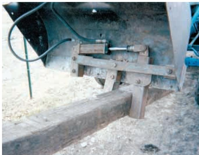
Bucket-mounted post gripper made it easy for Roger Holcomb to build a railroad tie fence by himself.
