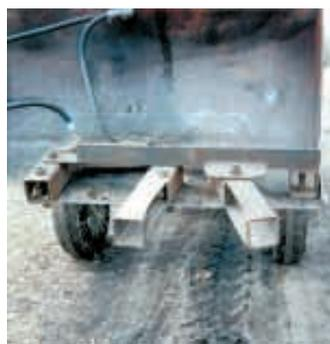
Two 3-ft. lengths of steel tubing act as grapple "fingers", one of which pivots back and forth (above). Hydraulic cylinder fastens to bottom of bucket.
