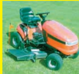
It's a lot safer than bending down to raise the discharge chute by hand, or removing it entirely. It also makes it easier to mow tall grass without making windrows or plugging up the chute. Many newer riding mowers are equipped with an automatic shutoff switch under the seat, so if you bend down you can accidentally stall the mower.
