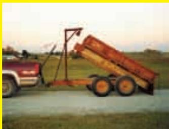
frame of a fertilizer spreader equipped with 10-ft. long I-beams. The front part of the bed is raised or lowered by an electric winch mounted in my pickup bed. A cable with eye goes from the dump bed, up over a pulley on an A-frame at the front of the trailer to the winch. (Ben D. Marek, 3885 Indian Road, New Ulm, Texas 78950)
