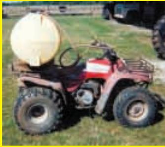
trols the flow to the boom and another one controls the flow to a hand wand that's attached to a 15-ft. hose. The rig has an 8-ft. long boom equipped with seven nozzles, and an off-center flat spray nozzle that's used to spray along fence rows. The nozzle covers a 68-in. wide area so it can spray both sides of the fence in one pass.
