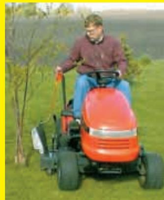
Our new attachment for riding mowers lets you lift the discharge chute up out of the way on-the-go for easier trimming and parking in tight areas.
