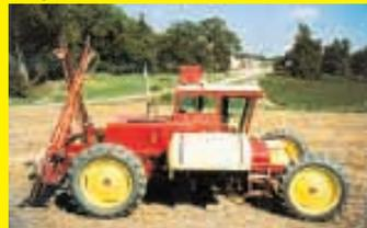
I've used my combine sprayer for three years. It costs very little to maintain, and the diesel engine is fuel efficient. I spent about \$5,000 to build it. I saved that much just in one season by not having to hire a custom spraying service. And, I can shop for chemicals and do my own application when I need to without having to wait for someone else to do the job for me.
