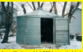
I modified an old 1,350-bu. grain bin to store wood for my outdoor furnace. I cut out a pair of doors that measure 6 ft. 4 in. wide. I used 2-in. wide, 5/32-in. thick
