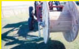
secure by a length of chain. The spool can handle up to a half mile of wire at a time. (Dwight Ruhlen, 2591 Halcyondale Rd., Sylvania, Ga. 30467 ph 912 863-4398)
