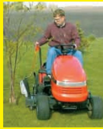
Our new attachment for riding mowers lets you lift the discharge chute up out of the way on-the-go for easier trimming and parking in tight areas.
