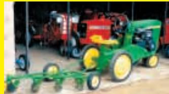
Thanks for the story on the motorized pedal tractor that I built for my grand kids (Vol. 24, No. 6). The tractor is built out of a Deere 20 series pedal tractor which I completely restored. A 3 1/2 hp Briggs and Stratton gas engine direct-drives a centrifugal clutch which chain-drives the rear axle.
