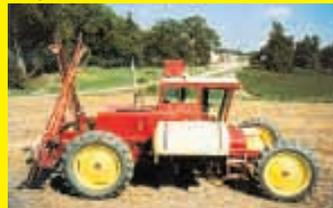
I've used my combine sprayer for three years. It costs very little to maintain, and the diesel engine is fuel efficient. I spent about \$5,000 to build it. I saved that much just in one season by not having to hire a custom spraying service. And, I can shop for chemicals and do my own application when I need to without having to wait for someone else to do the job for me.
