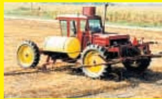
I converted an old Massey 750 combine into a low-cost, self-propelled sprayer equipped with rear wheel drive and front axle steering. The machine drives and steers off the front axle, just like a tractor, so it turns sharp and is easy to maneuver. It has a 60-ft. boom and a pair of 300-gal. tanks and rides on 18.4 by 38 wheels. Its low center of gravity helps keep it stable on sidehills.
