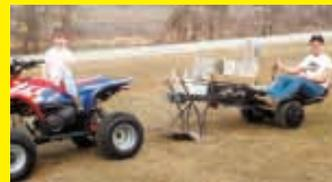
hp engine on back to pull the weight transfer box up the frame, which works via a belt and pulley system. I mounted a seat on one side at the back where I sit while running the engine and operating a lever that controls the weight transfer box. Cement blocks provide the weight.
