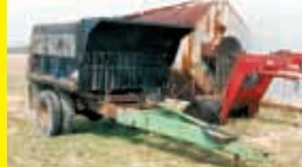
blown engine. The rear end, box, and dump hoist were in good shape. The long planter tongue gives the dump trailer plenty of maneuvering room behind a tractor. (**Dean Nixon, 10544 Piasa Rd., Medora, Ill. 62023 ph 618 729-3865**)
