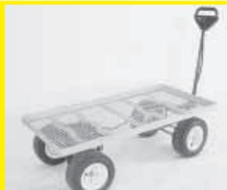
A friend and I have come up with what we call the Pack Rat. It's an electric-powered wagon that's really generating a lot of interest. It rolls on four pneumatic 12-in. turf tires and has an angle iron frame. It has removable sides and measures 2 by 4 ft. Recommended weight capacity is 500 lbs. Power is provided by an electronic-controlled transaxle equipped with a 24-volt smart charger (included). The 12-volt gel cell batteries are wired in series. The unit will charge overnight.
