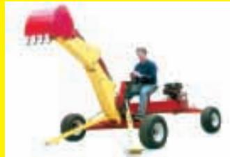
motor and rides on balloon tires that are highway-rated. Support legs provide an 8-ft. wide base. Boom arms are laser cut from heavy plate steel. Bucket has replaceable teeth. You can use the bucket to move the unit along when in use.
