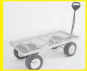
A friend and I have come up with what we call the Pack Rat. It's an electric-powered wagon that's really generating a lot of interest. It rolls on four pneumatic 12in. turf tires and has an angle iron frame. It has removable sides and measures 2 by 4 ft. Recommended weight capacity is 500 lbs. Power is provided by an electronic-controlled transaxle equipped with a 24-volt smart charger (included). The 12-volt gel cel batteries are wired in series. The unit will charge overnight.
