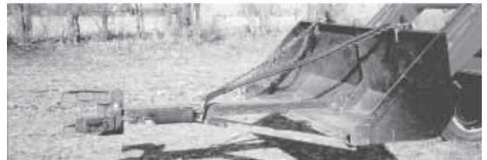
Unit is bolted to the end of a steel tube and extends about 7 ft. in front of loader bucket.
