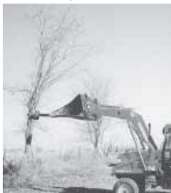
Tractor driver clamps the "claw" around tree while another person uses a chain saw to cut tree off.
