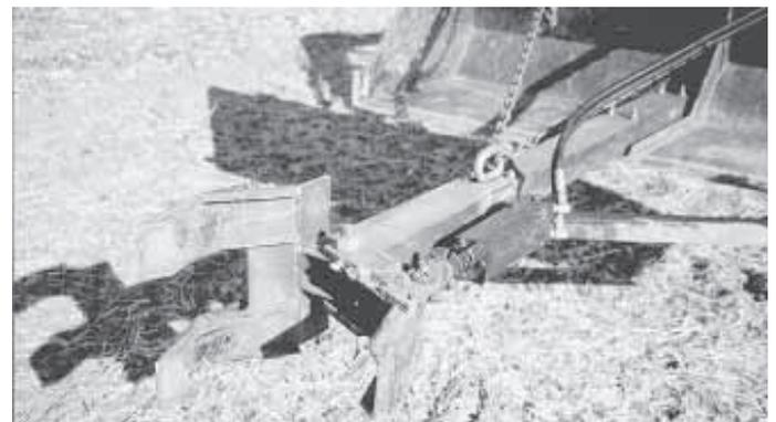
"Claw" consists of two stationary fingers and a single, movable finger connected to a hydraulic cylinder.
