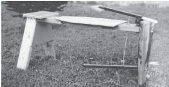
Foot-operated lever applies downward pressure to hold fish in place.
