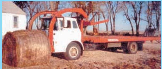
Bale-hauling truck designed by Richard and Dennis Weber is built around a 1972 Chevrolet C-50 cab-over truck. It can load up 10 big round bales on-the-go.
