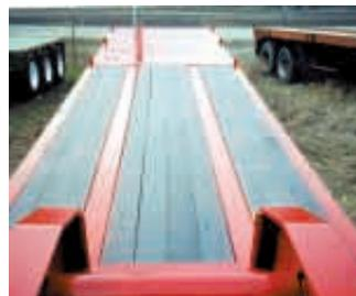
"Rubber" is made of ground-up scrap tires and recycled plastic. Here it was used to make a trailer floor.
