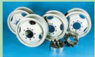
Kit includes new dual-style wheels and adapters that let you mount duals onto your existing axle with no modifications. sources say even the high end kits with aluminum wheels are under \$1,000.
