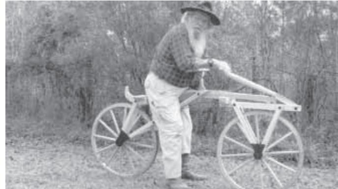
Chuck Smart built this replica of the first bicycle ever built. It has no pedals. You just run and coast.
