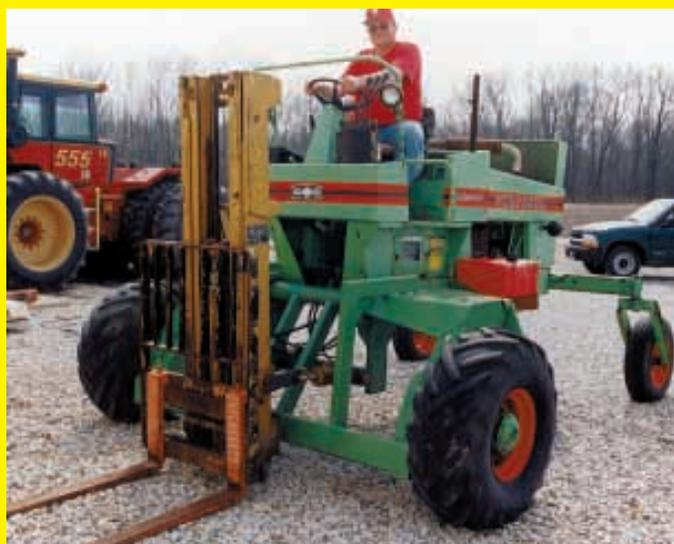
To make their Owatonna swather more useful during the off season, Tim and Tom Nelson mounted a 3-stage forklift mast on front. A hydraulic cylinder mounted underneath tilts the frame forward and back.
