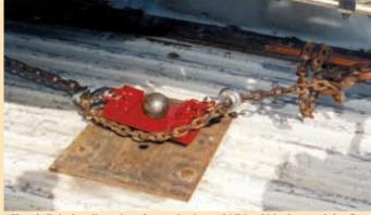
"Clamshell tie-down" consists of a couple pieces of 1/2-in. thick plate steel that fit on either side of the ball hitch and hook together with a lynch pin.
