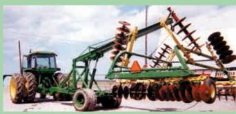
Loader tows behind a tractor and is hydraulically raised and lowered by an 18-ft. boom.
