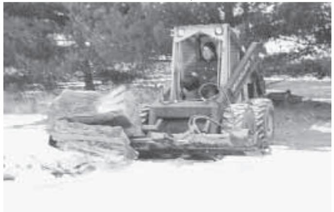
**Unit can split logs up to 46 in. long and any diameter.**
