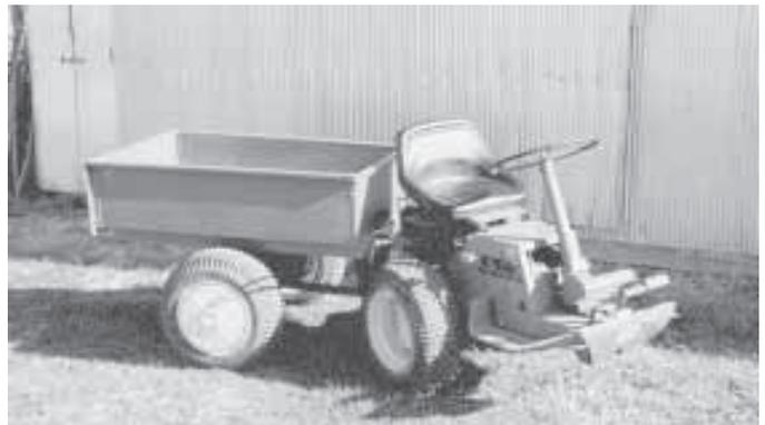
**To make his utility vehicle, Stanley Byerly joined a dumping yard trailer to an old Deere 72 front deck riding mower.**
