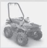
driver's head. The bar is made from steel tubing and bolts onto the rear rack. The bulbs are said to deliver up to three times as much light as standard high intensity bulbs found on most ATV's, and are also equipped with an optical lens. The result is a 20-degree wide horizontal beam of light with up to 2,600 ft. of reflective range. The lights are turned on or off with a switch. All wiring is included.
