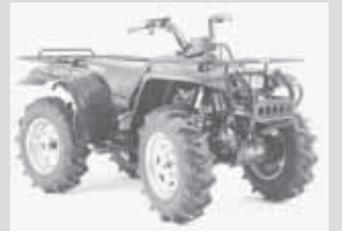
**Farm AG Kit** - This "kit" consists of super-tall 27-in. tires that turn your 4-WD ATV into a mini tractor, says the company. The 4-ply tires have self-cleaning "super lug" tread for slow-speed agriculture usage. Works great in very wet conditions. According to the company, no other ATV-type tire can match this tire's pulling power.
