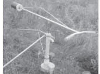
Manual pump works something like an old fashioned well pump and is made from two pieces of PVC pipe.
