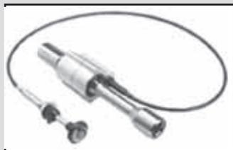
ATV's allows you to switch from 4-WD to 2-WD and back again, all on-the-go. Disengaging the front wheels makes the ATV a lot easier to steer, says the company. It also saves wear and tear on front-end parts. The entire unit replaces the ATV's front driveshaft and is controlled by a spring-loaded cable.
