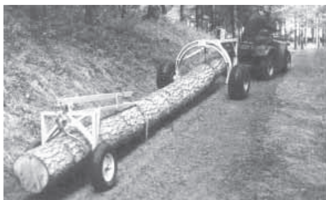
For longer logs a second arch can be used on back, allowing you to carry both ends of log. A hand-pushed model for smaller logs is also available.
