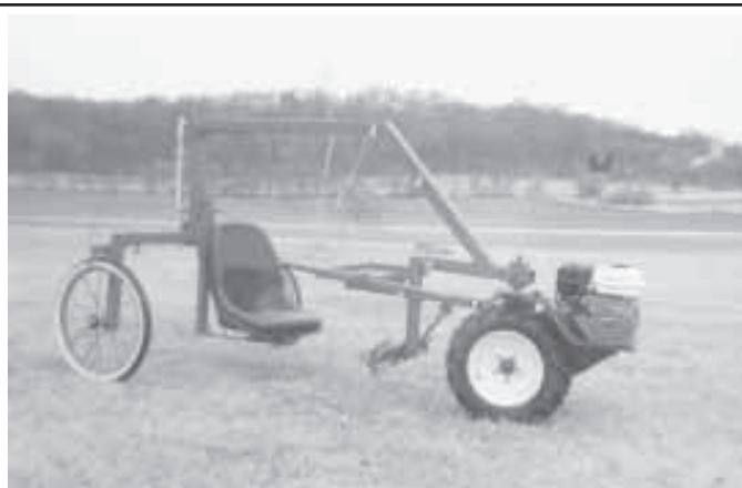
Junior Gurgel built a lot of adjustable features into this 3-wheeled picker. It's powered by a 5 1/2 hp Honda gas engine that belt-drives the front wheel.
