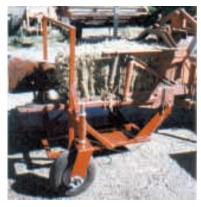
Tag-along bale scale rides on two small wheels directly behind bale chamber In-cab monitor, above,
