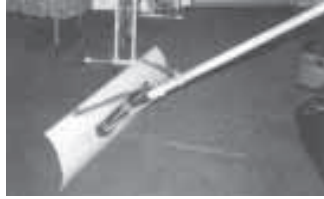
Howe modified scraper so handle runs into back of blade, braced by angled struts.
