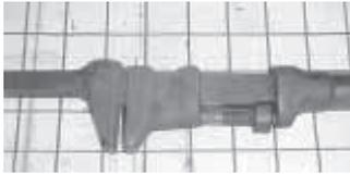
"I also added an extra handle to the top of an adjustable pipe wrench. I just welded it in place. It's handy for getting a good grip for turning."
