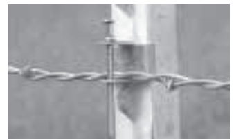
Crimper attaches clips onto T-posts.
