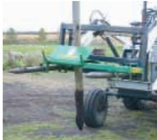
**When operator lifts loader and tips it back, edge of gate bites into side of post to pull it out of ground.**
