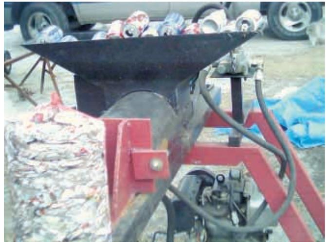
Log splitter attachment has a hopper that allows it to crush a bunch of cans at once, rather than one at a time like most crushers.
