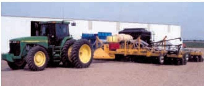
Planter's fitted with a Yetter Seed Jet that loads and unloads the seed hopper.
