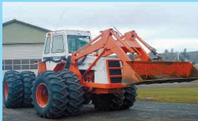
Ron Kile cut this tractor in half to convert it to articulated steering. He built a front-end loader to fit the big tractor.
