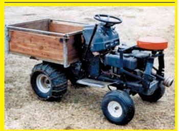
I made this wood hauler from an old riding lawn mower. The box trips to dump the wood. Works great and I can take it right
